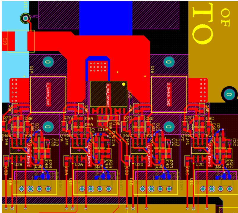
Figure 3.14: 2D layout of a CSI leg.
