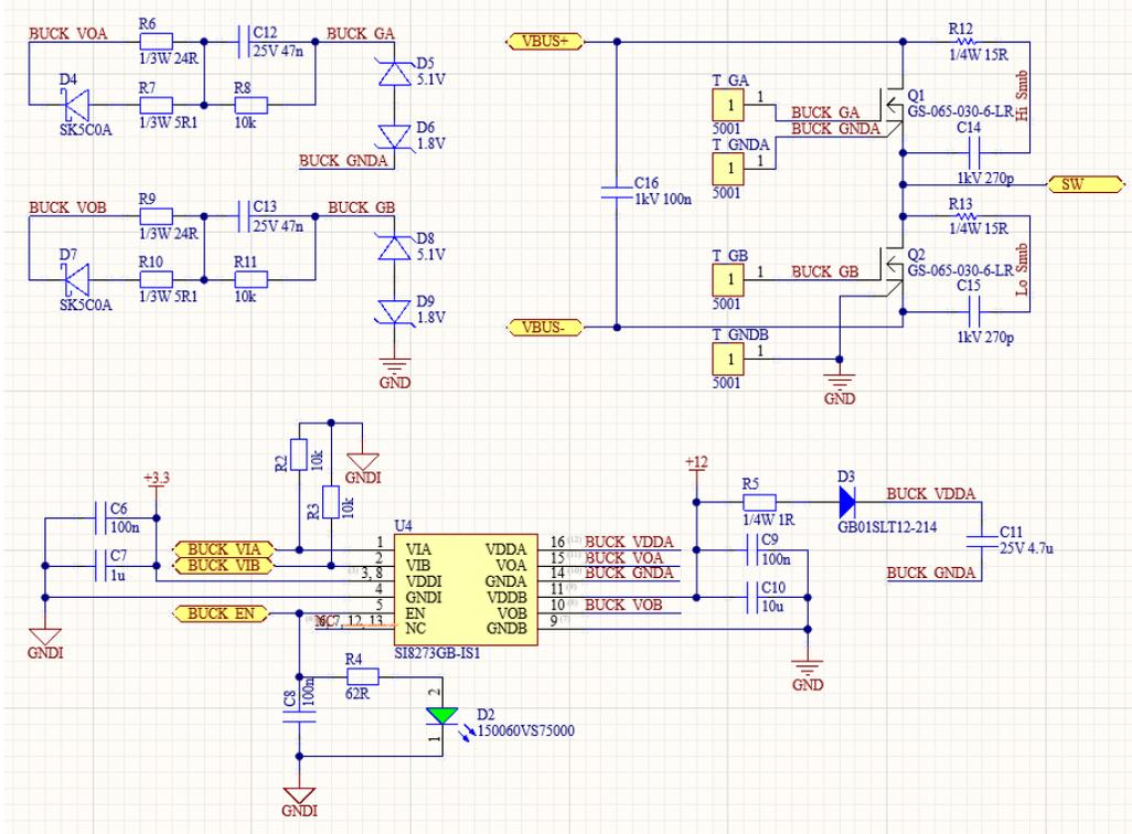
Figure 3.3: Schematic of the synchronous buck converter.
