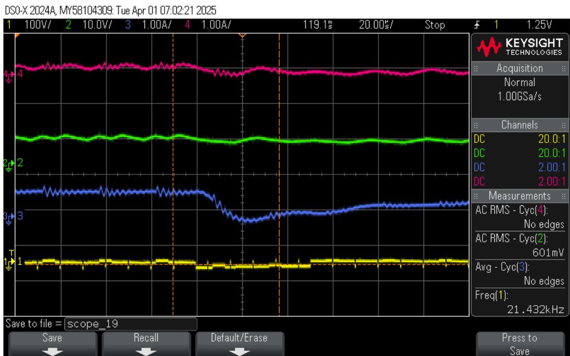
Figure 4.9: Zoom into Figure 4.8 to observe buck response to  $I_{dc}$ .
