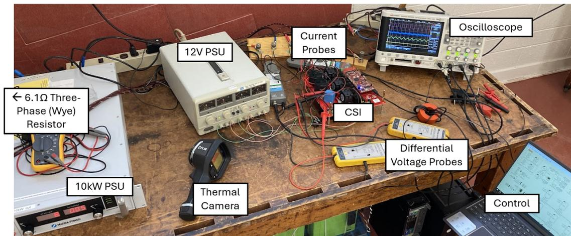
Figure 4.2: Experimental setup for driving a three-phase resistive load.
