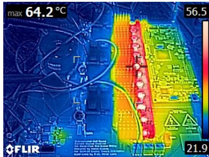
Figure 4.11: Thermal measurement of the prototype board at  $I_{ref} = 700$  mA and  $f_s = 40$  kHz under buck converter operation.
