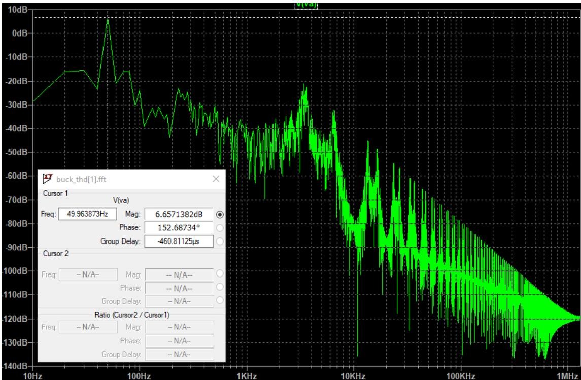
Figure 4.13: Fourier transform of  $V_{Cf,a}$  under buck converter operation from Figure 4.10.
