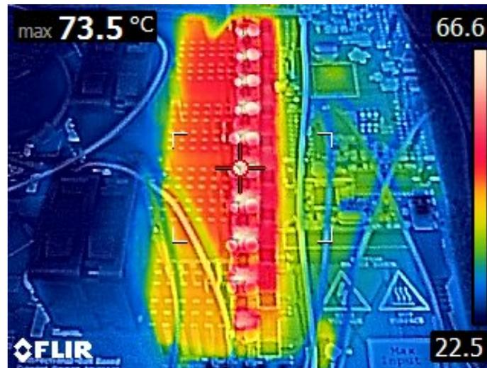
Figure 4.5: Thermal measurement of the CSI gate drivers and heatsinks at  $I_{dc} = 1$  A and  $f_s = 40$  kHz under constant current supply.
