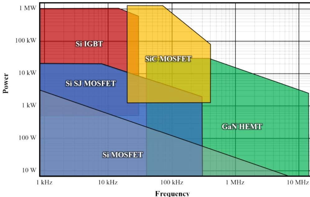
Figure 2.4: Frequency and power regions for different power semiconductor technologies [5].
