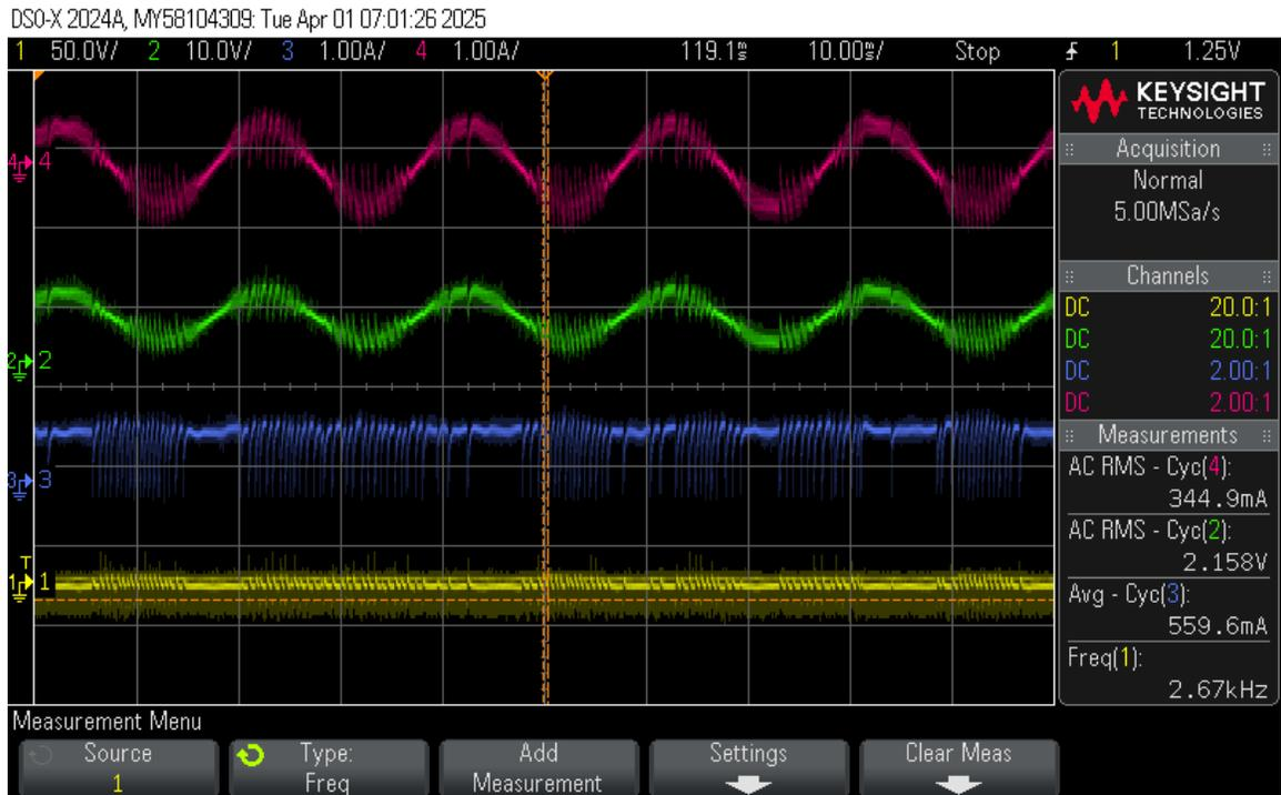
Figure 4.8: Phase A and input voltages and currents under buck converter operation with  $V_{in} = 13\text{ V}$  (yellow:  $V_{Ldc}$ , green:  $V_{Cf,a}$ , blue:  $I_{dc}$ , pink:  $I_{out,a}$ ).
