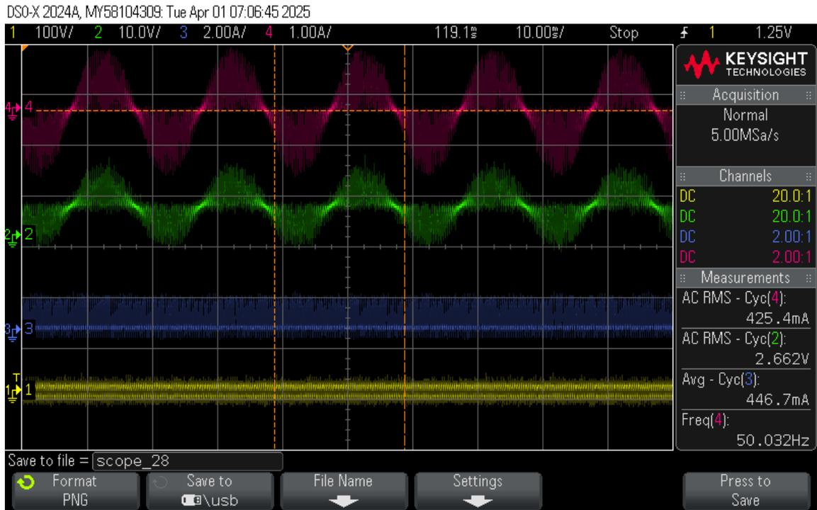
Figure 4.10: Phase A and input voltages and currents under buck converter operation with  $V_{in} = 20$  V (yellow:  $V_{Ldc}$ , green:  $V_{Cf,a}$ , blue:  $I_{dc}$ , pink:  $I_{out,a}$ ).
