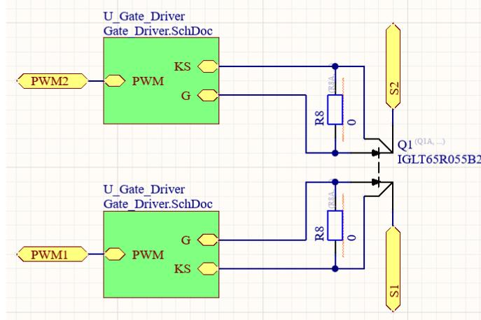
Figure 3.4: Schematic of the switch cell.
