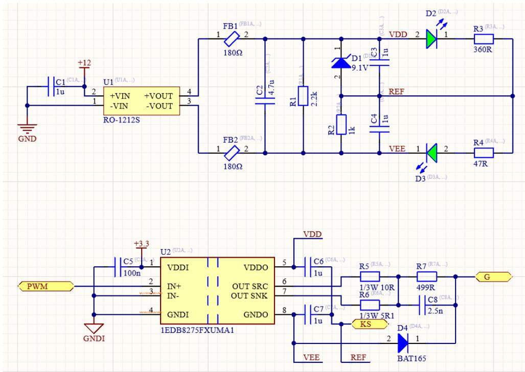
Figure 3.5: Schematic of the BD-GaN gate driver.
