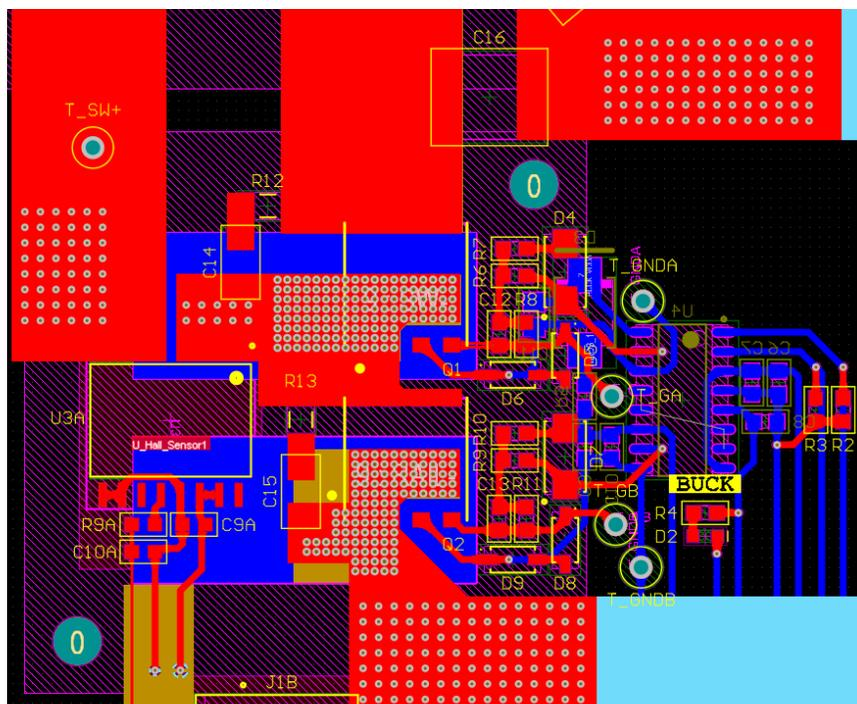
Figure 3.12: 2D layout of synchronous buck converter.
