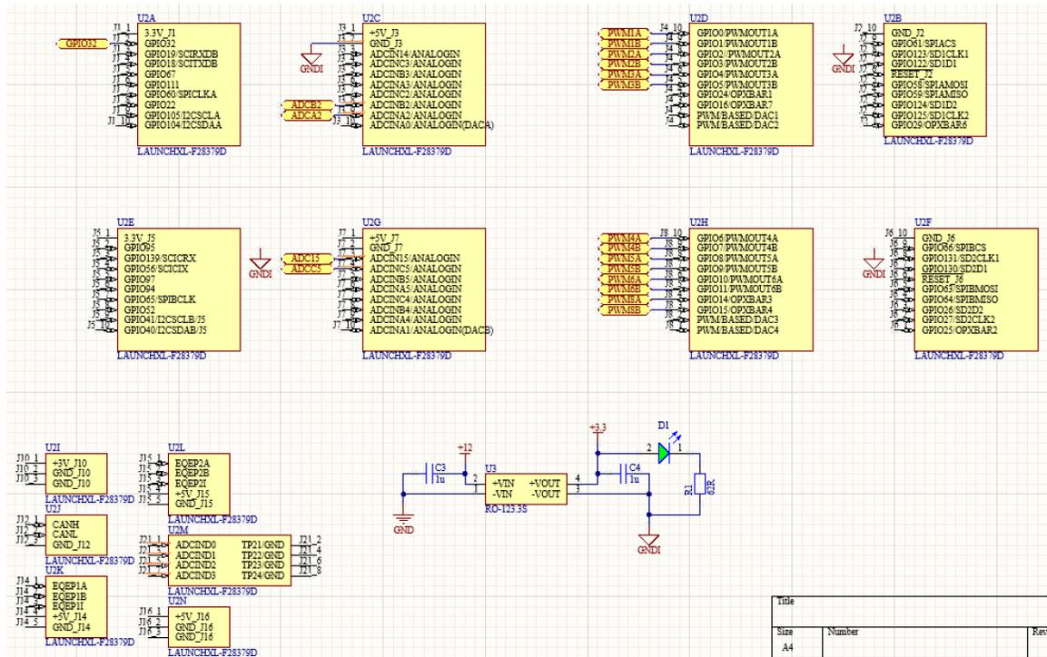
Figure 3.7: Schematic of the DSP signals and power.
