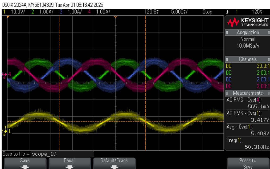
Figure 4.3: Three-phase output of the prototype board under constant current supply at  $I_{dc} = 1$  A (yellow:  $V_{Cf,a}$ , green:  $I_{out,a}$ , blue:  $I_{out,b}$ , pink:  $I_{out,c}$ ).
