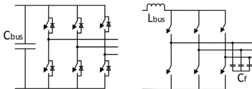
Figure 2.3: Basic topologies of a three-phase VSI (left) and CSI (right) [4].
