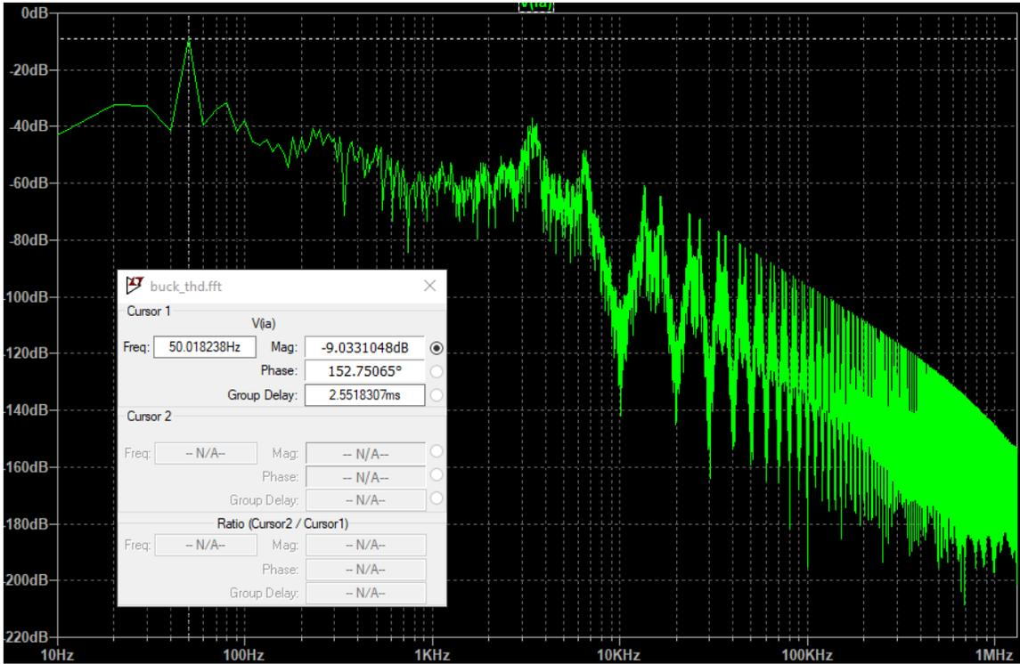
Figure 4.12: Fourier transform of  $I_{out,a}$  under buck converter operation from Figure 4.10.
