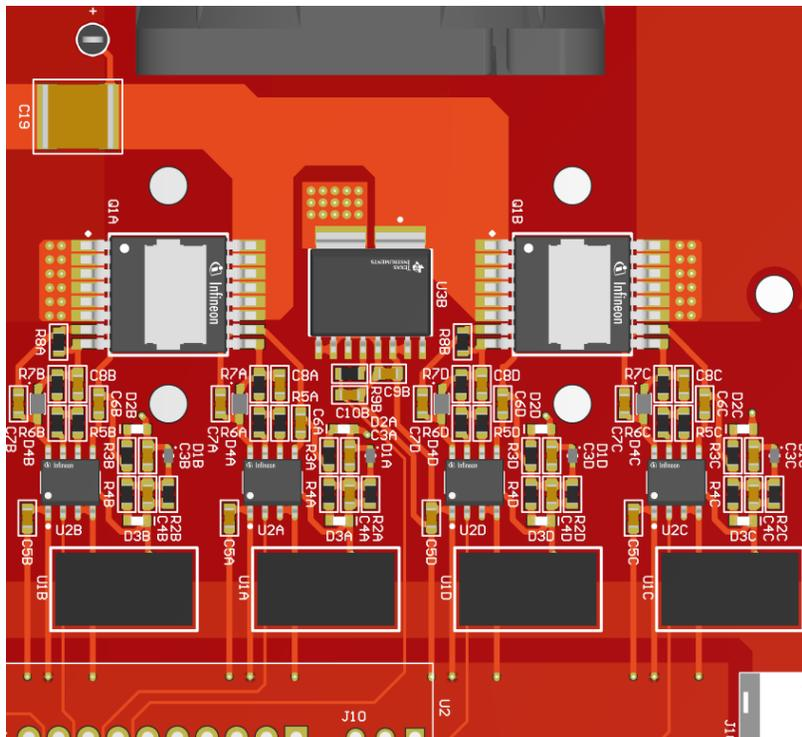
Figure 3.15: 3D orthographic layout of a CSI leg (heatsink and DSP 3D bodies removed).
