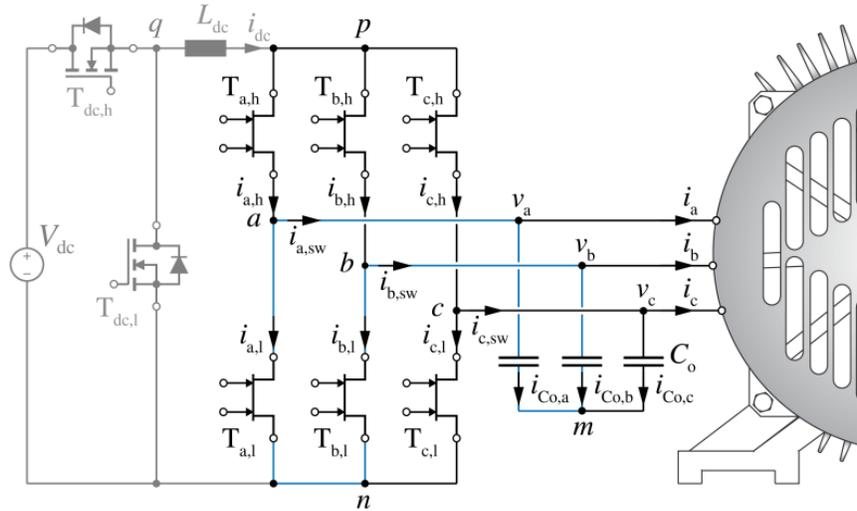
Figure 3.1: The CSI architecture to be implemented [7].
