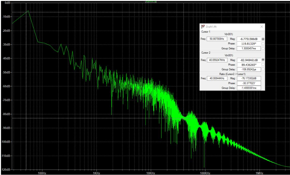
Figure 4.6: Fourier transform of  $I_{out,a}$  under constant current supply from Figure 4.4.
