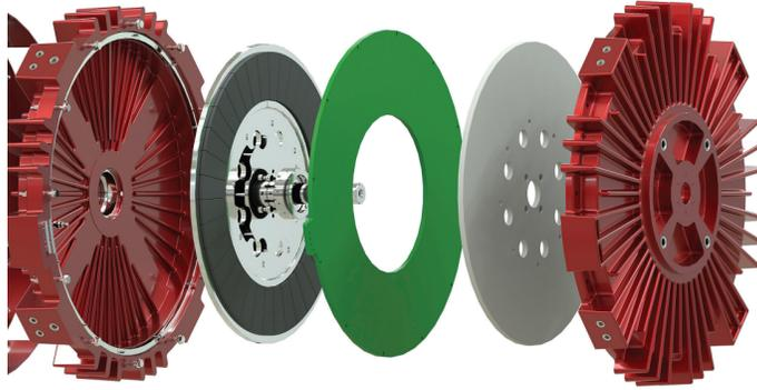
Figure 2.2: Exploded view of *Infinitum Electric*'s PCB-stator motor, showing the back motor housing, back rotor, PCB stator, front rotor, and front housing (left to right) [3].
