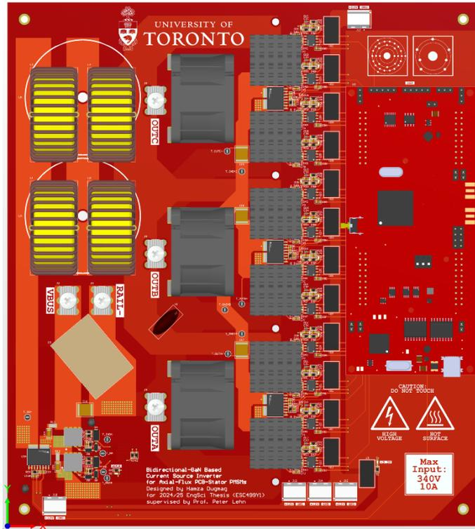
Figure 3.10: 3D orthographic layout of the entire top layer.
