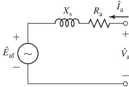
Figure 2.1: Circuit model of a synchronous motor [2].
