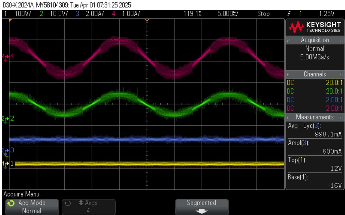
Figure 4.4: Phase A and input voltages and currents under constant current supply at  $I_{dc} = 1$  A (yellow:  $V_{Ldc}$ , green:  $V_{Cf,a}$ , blue:  $I_{dc}$ , pink:  $I_{out,a}$ ).
