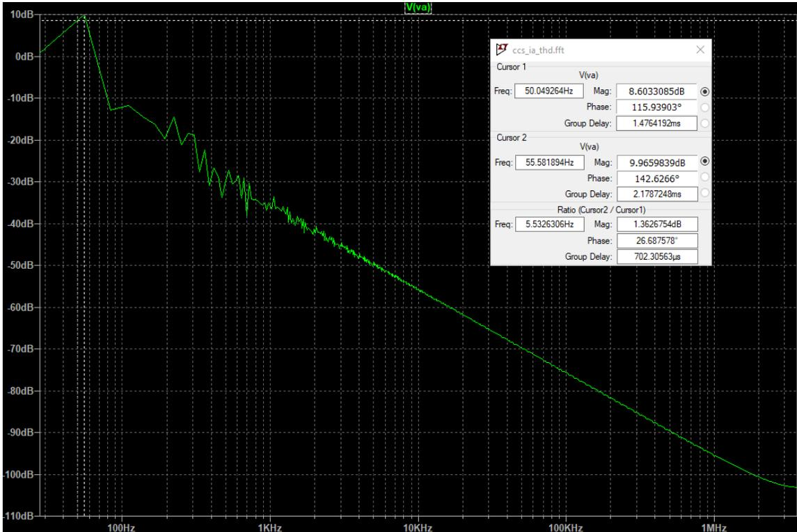
Figure 4.7: Fourier transform of  $V_{Cf,a}$  under constant current supply from Figure 4.4.
