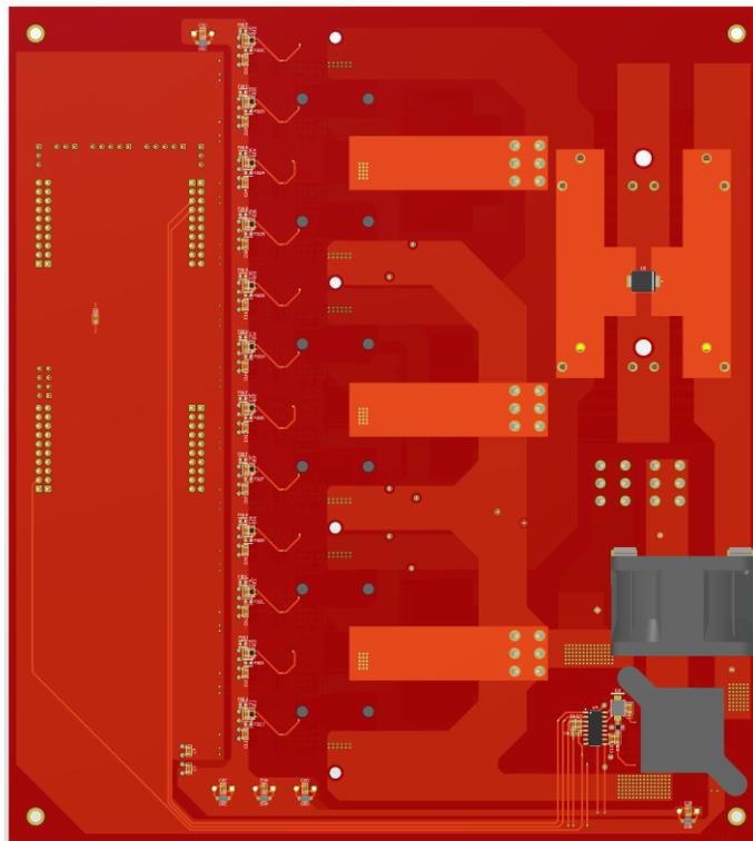
Figure 3.11: 3D orthographic layout of the entire bottom layer.
