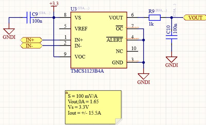
Figure 3.6: Schematic of the Hall sensor.
