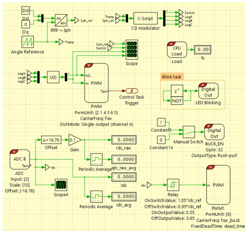
Figure 3.17: PLECS firmware for the C2000 DSP for CSI and buck control.
