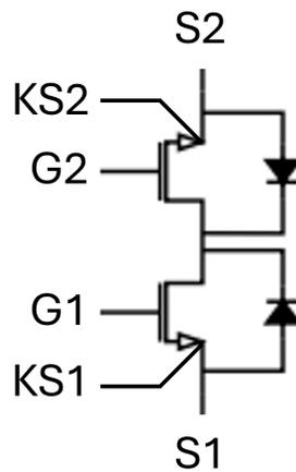
Figure 2.6: Effective equivalent circuit of the IGLT65R055B2.
