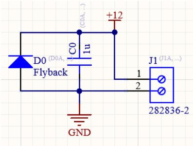
Figure 3.8: Schematic of the 12 V auxiliary supply.
